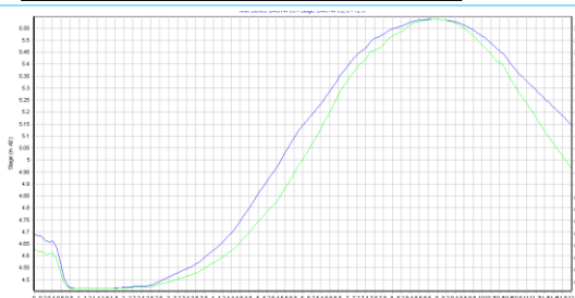
Flow (green) and Stage(blue) through culvert DNG147C3
