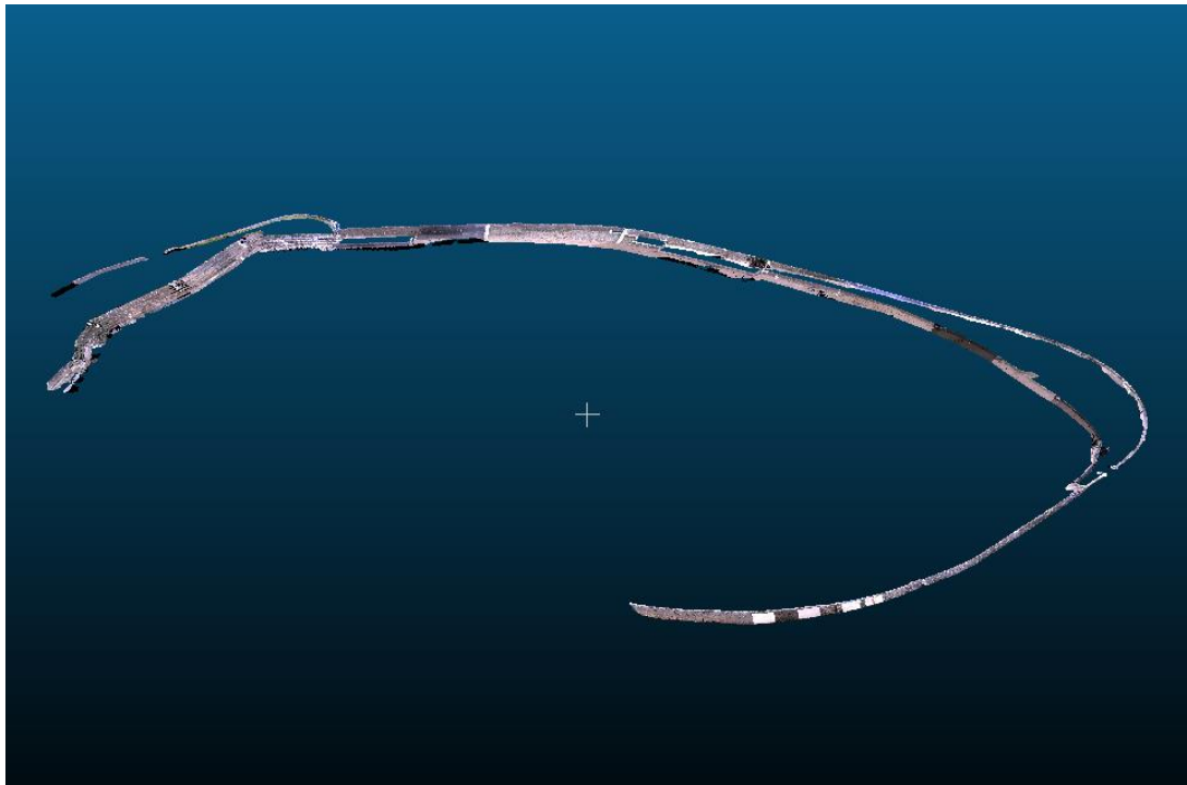
Figure 2-11: Laser Survey of Sea Wall
