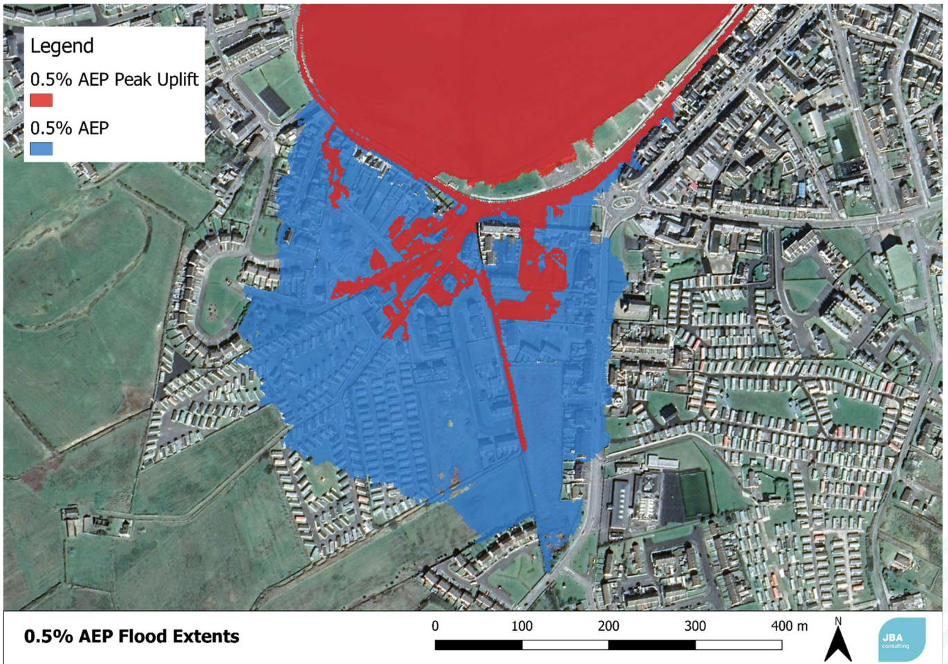
Figure 5-2: 0.5% AEP comparison of wave setup
