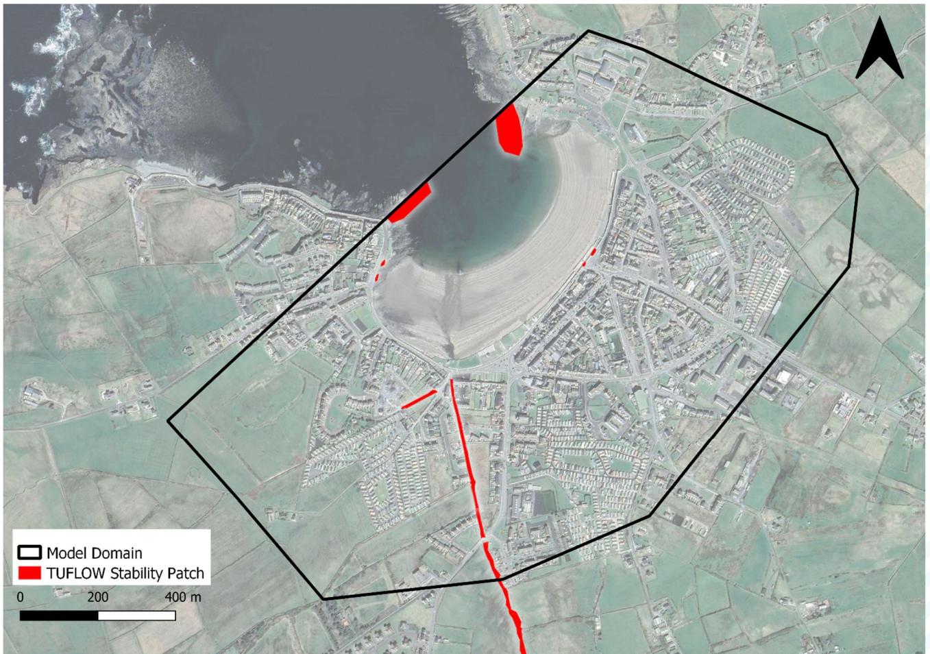
Figure 2-9: Location of increased topographic roughness for model stability
