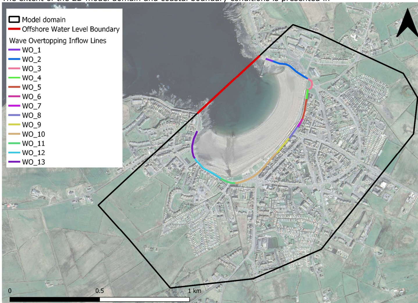
Figure 2-5. The model was constructed using a 2m resolution fixed grid suitable to pick out the key overland coastal flood flow paths.
