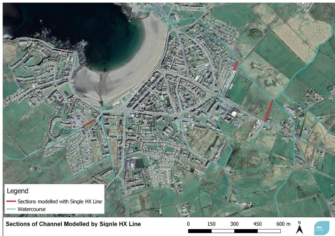
Figure 3-12: Sections of Channel Modelled with single HX line
